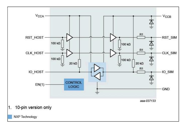
View additional information for SIM Card Interface Level Translator with EMI Filter and ESD Protection.
