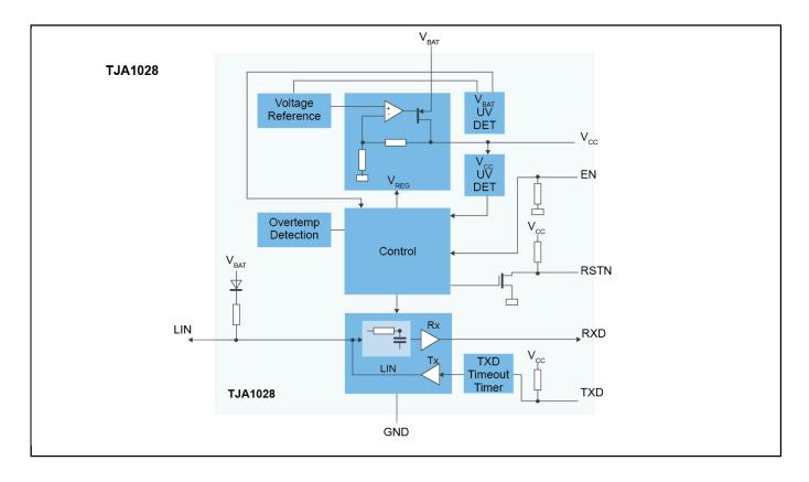
View additional information for LIN Transceiver with Integrated Voltage Regulator.
