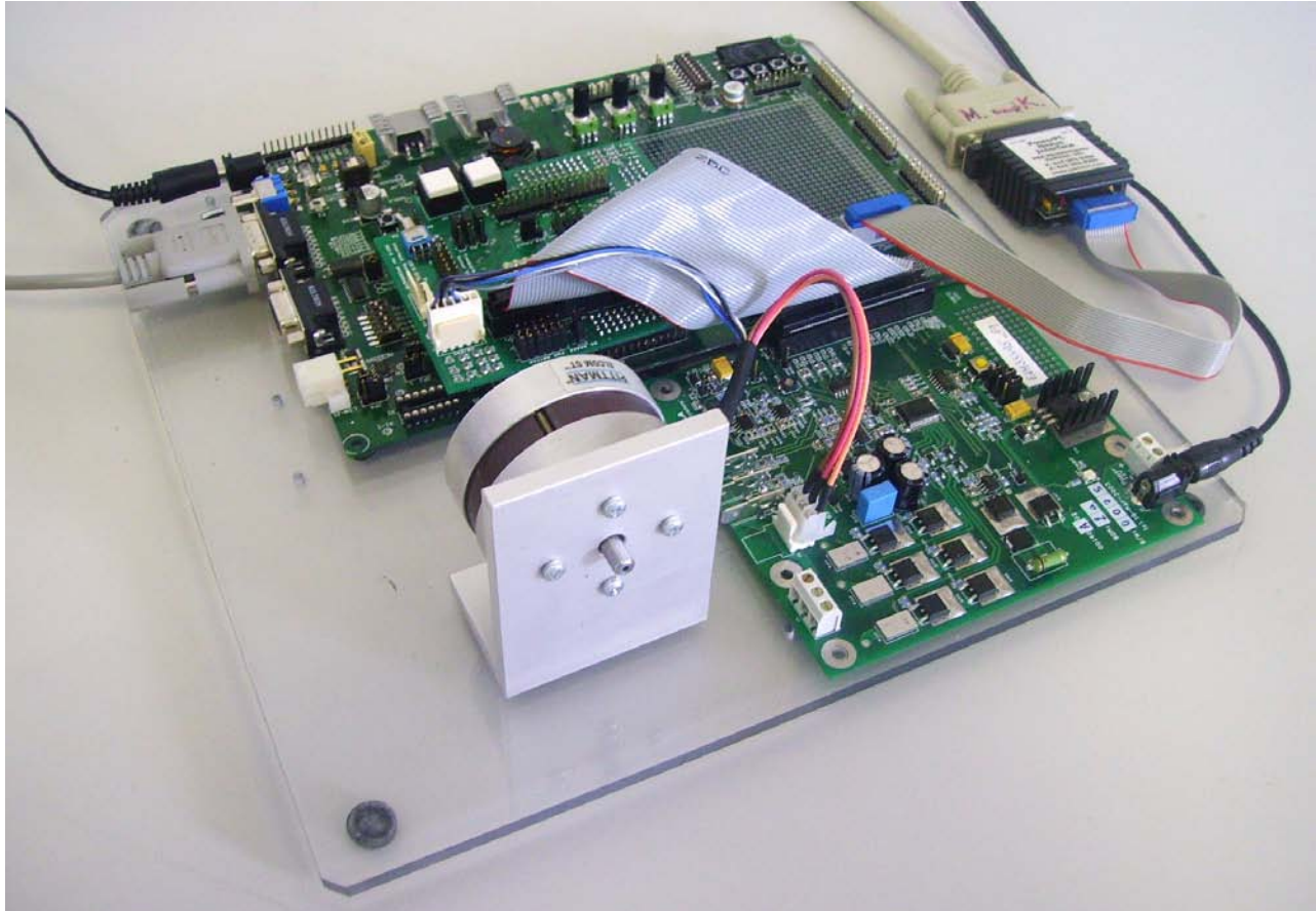
Figure 1. Using MPC5554DEMO, 33395 Evaluation Motor Board, and Pittman BLDC Motor
