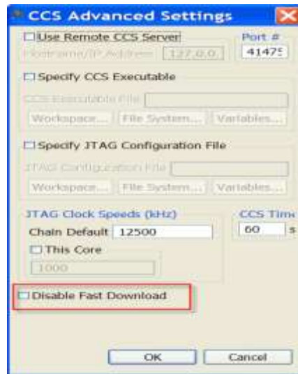
Figure 47. Non-RSE CodeWarrior Project, Disable Fast Download Setting.
