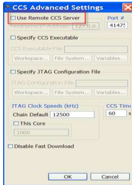
Figure 36. Non-RSE CodeWarrior Project, Use CCS Remote Server Setting.
