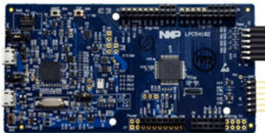
Figure 5. LPCXpresso 54102 board as USB-to-SPI tool
