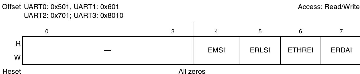
Figure 13-7. Interrupt Enable Register (UIER)
