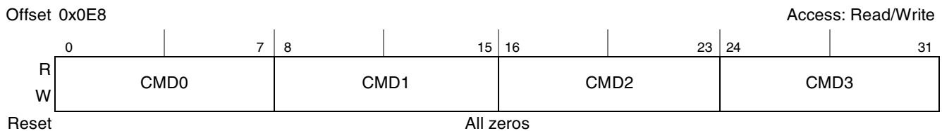
Figure 9-22. Flash Command Register
