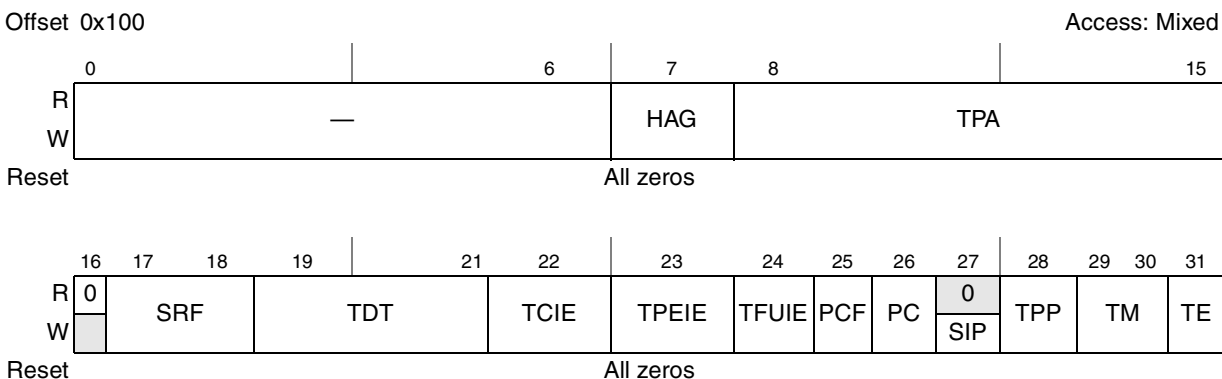
Figure 14-18. Transmitter Control Register (FIRITCR)
