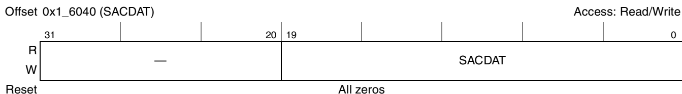
Figure 16-30. SSI AC97 Command Data Register (SACDAT)
