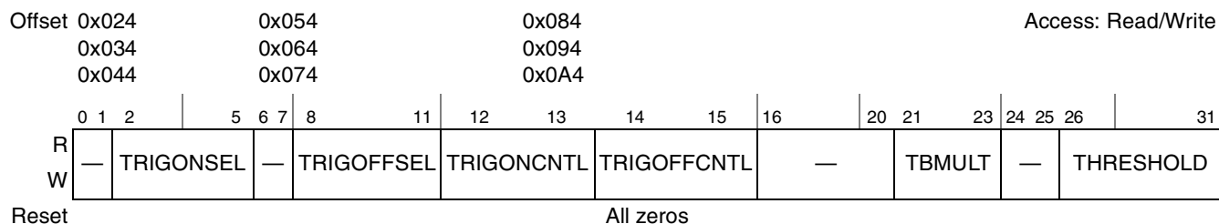
Figure 24-6. Performance Monitor Local Control Register B (PMLCB1–PMLCB9)
