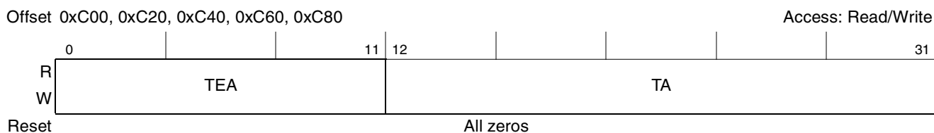
Figure 20-6. PCI Outbound Translation Address Registers (POTAR n )
