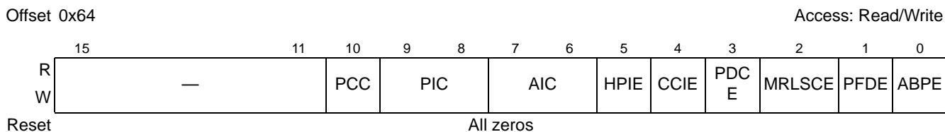
Figure 17-103. PCI Express Slot Control Register
