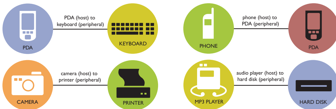
Figure 3: OTG enables point-to-point connectivity between peripherals without a traditional PC host.
