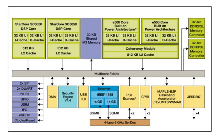
View additional information for QorIQ® Qonverge BSC9132 Dual-Core Processor and Dual-Core DSP.
