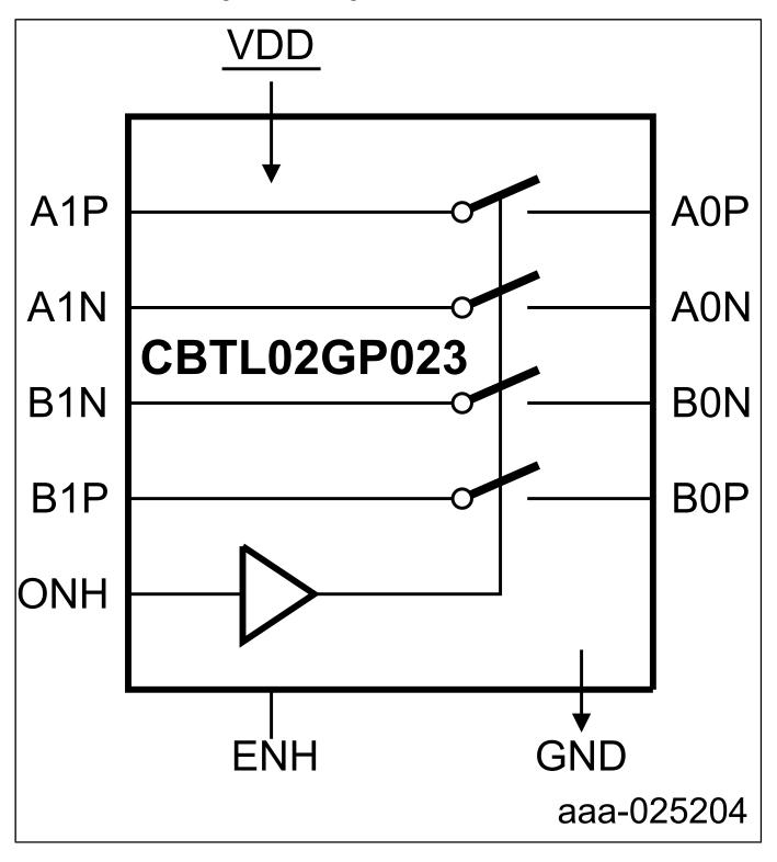
View additional information for 5 Gbps Rail-to-Rail Low-Insertion Loss Switch.
