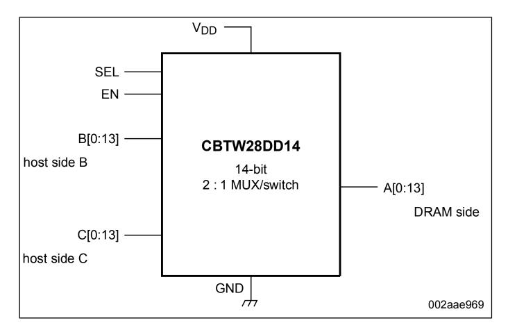
View additional information for 14-Bit Bus Switch/Multiplexer for DDR2/DDR3/DDR4 Applications.
