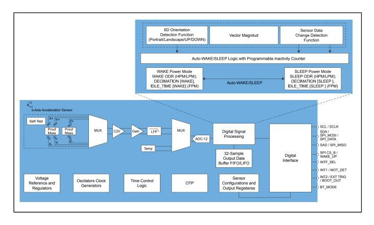
View additional information for ±2g/±4g/±8g/±16g, Low Power 12-Bit Digital Accelerometer.
