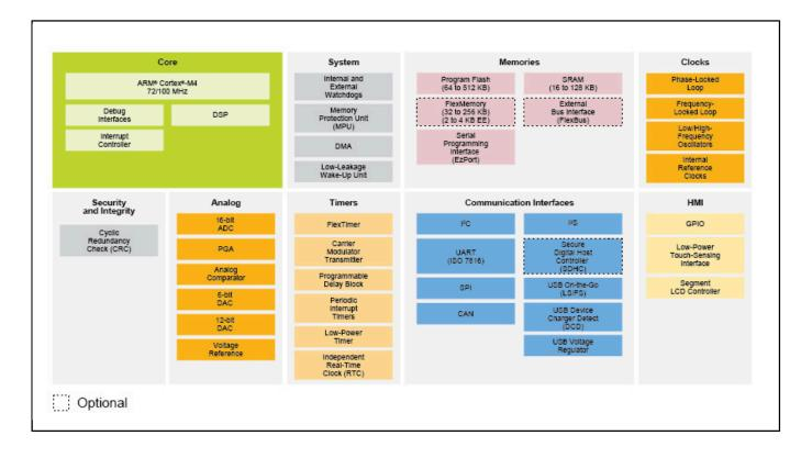
View additional information for Kinetis® K40-100 MHz, Mixed-Signal Integration Microcontrollers (MCUs) based on Arm® Cortex®-M4 Core.
