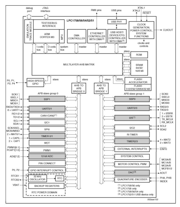
View additional information for Scalable Mainstream 32-bit Microcontroller (MCU) based on Arm® Cortex®-M3 Core.
