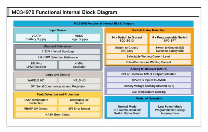
View additional information for Switch Detection Interface, 22 I/Os, Programmable Wetting Current, Temp Sensor, 3.3 V / 5.0 V SPI.
