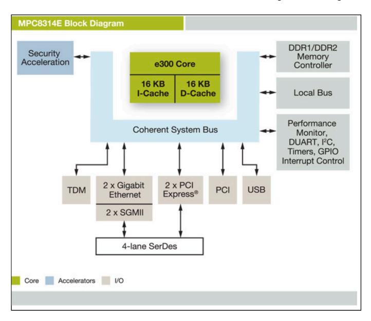
View additional information for Low-Power PowerQUICC® II Pro Processor with DDR2, TDM, PCI, PCI Express, 1 GB Ethernet, Security, USB.
