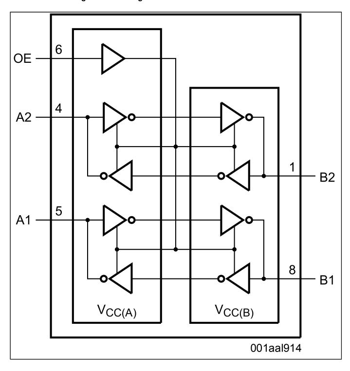
View additional information for Dual-Supply Translating Transceiver (Auto-Direction Sensing, Three-State).
