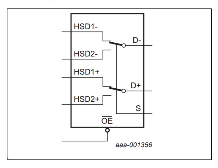
View additional information for Dual High-Speed USB 2.0 Double-Pole Double-Throw Analog Switch.
