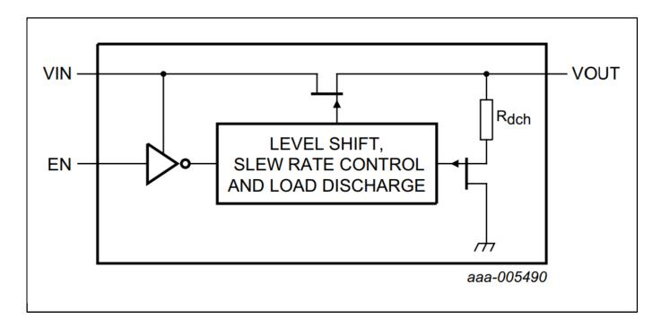
View additional information for Logic-Controlled High-Side Power Switch.
