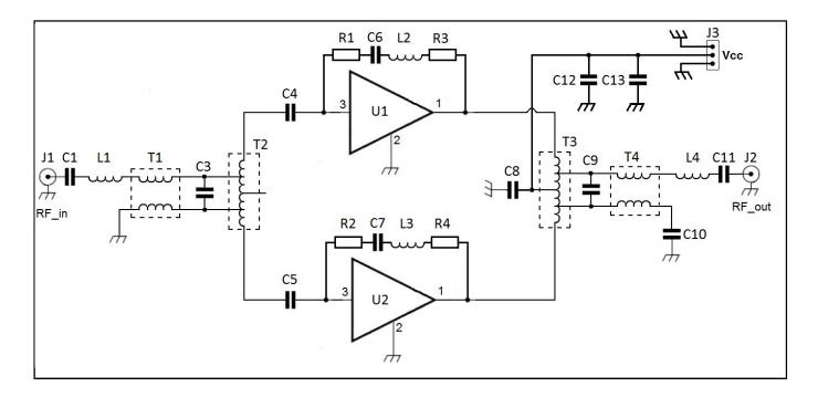
View additional information for Demo Board for BGA3018, 40 MHz to 1006 MHz Push-Pull Amplifier Application.
