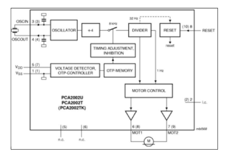
View additional information for 32 KHz Watch Circuit with Programmable Output Period and Pulse Width.
