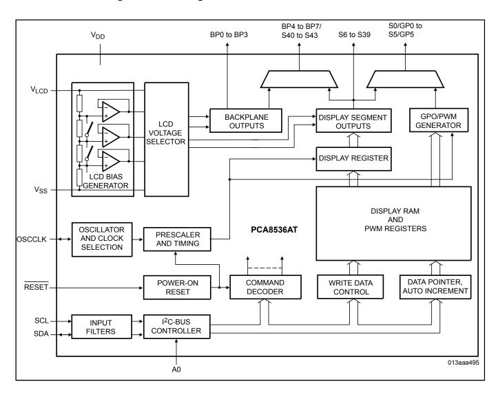
View additional information for Automotive LCD Driver for Low Multiplex Rates Including 6 Channel PWM Generator.
