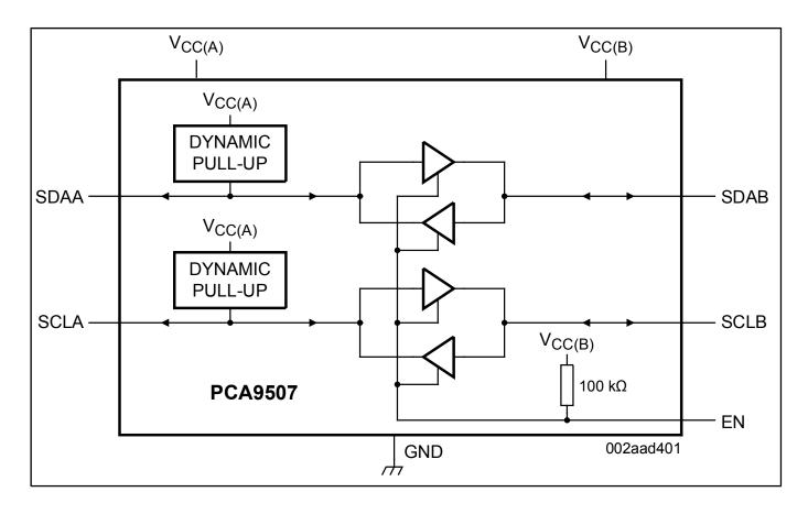
View additional information for Two-Wire Serial Bus Extender for HDMI DDC I2C-Bus and SMBus.
