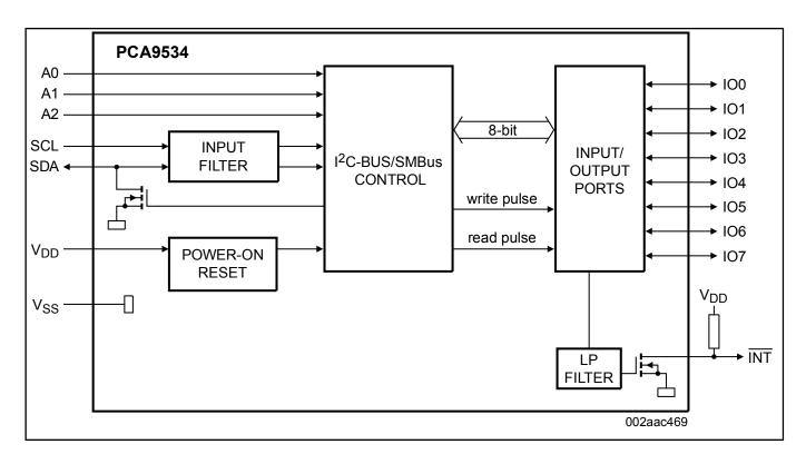
View additional information for 8-Bit I<sup>2</sup>C-Bus and SMBus Low Power I/O Port with Interrupt.
