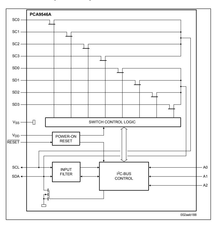
Block diagram: PCA9546ABS, PCA9546AD, PCA9546APW Block Diagram
