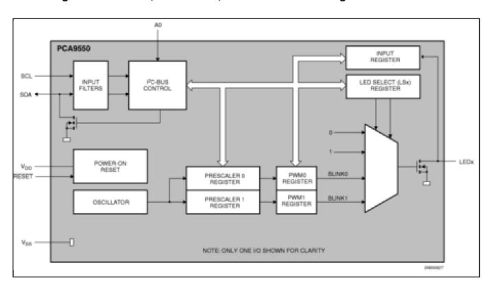
View additional information for 2-Bit I<sup>2</sup>C-Bus LED Driver with Programmable Blink Rates.
