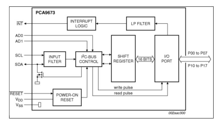
View additional information for Remote 16-Bit I/O Expander for Fm+ I2C-Bus with Interrupt and Reset.
