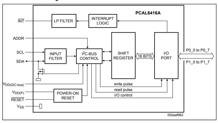
View additional information for Low-Voltage Translating 16-Bit I<sup>2</sup>C-Bus/SMBus I/O Expander.
