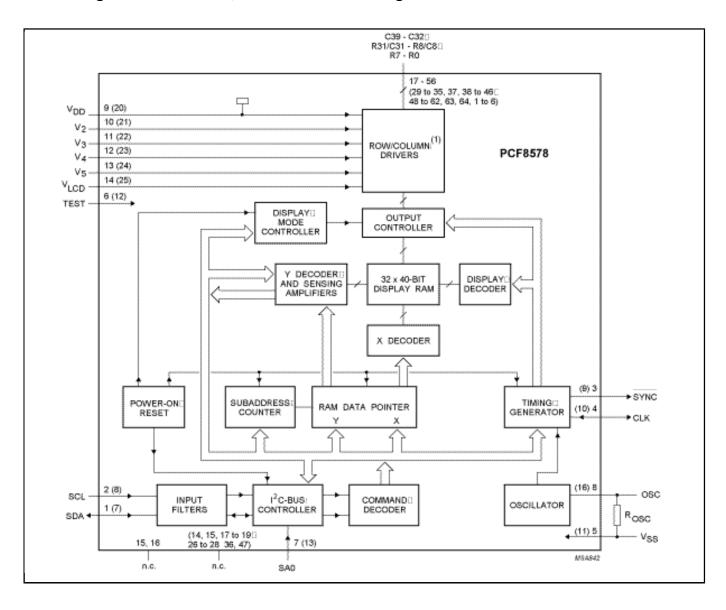
View additional information for LCD Row/Column Driver for Dot Matrix Graphic Displays.
