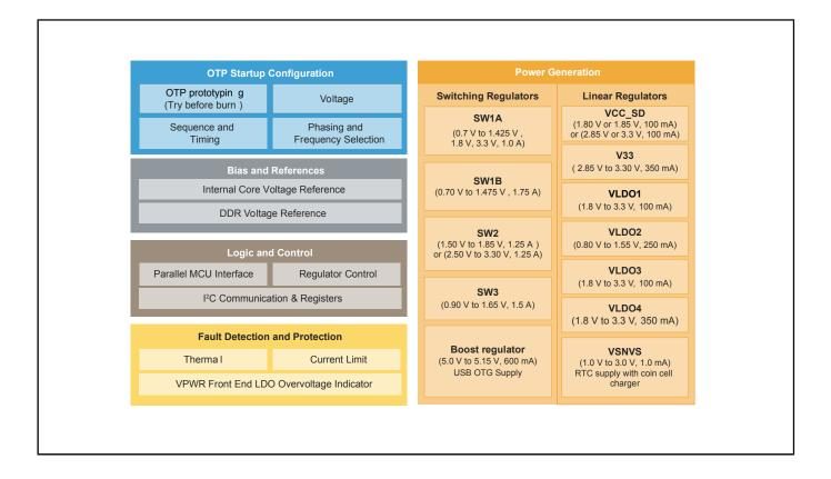
View additional information for 12-Channel Configurable PMIC for i.MX6 and i.MX7 Application Processors.
