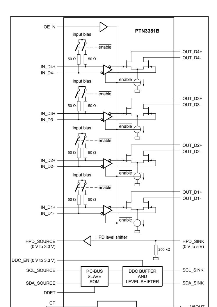
View additional information for Enhanced Performance HDMI/DVI Level Shifter with Voltage Regulator, Dongle Detect Support and Active DDC Buffer.
