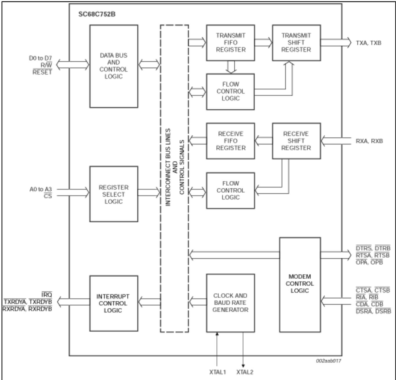
View additional information for [5 V](#), [3.3 V](#) and [2.5 V](#) dual UART, 5 Mbit/s (max.), with 64-byte FIFOs and 68 mode uP interfac.
