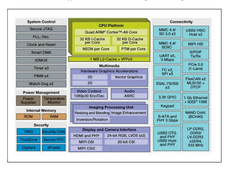
View additional information for i.MX 6Quad Processors - High-Performance, 3D Graphics, HD Video, Arm® Cortex®-A9 Core.
