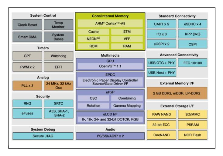
View additional information for Multimedia Applications Processors - Integrated Electronic Paper Display (EPD), High Performance, Arm® Cortex®-A8 Core.
