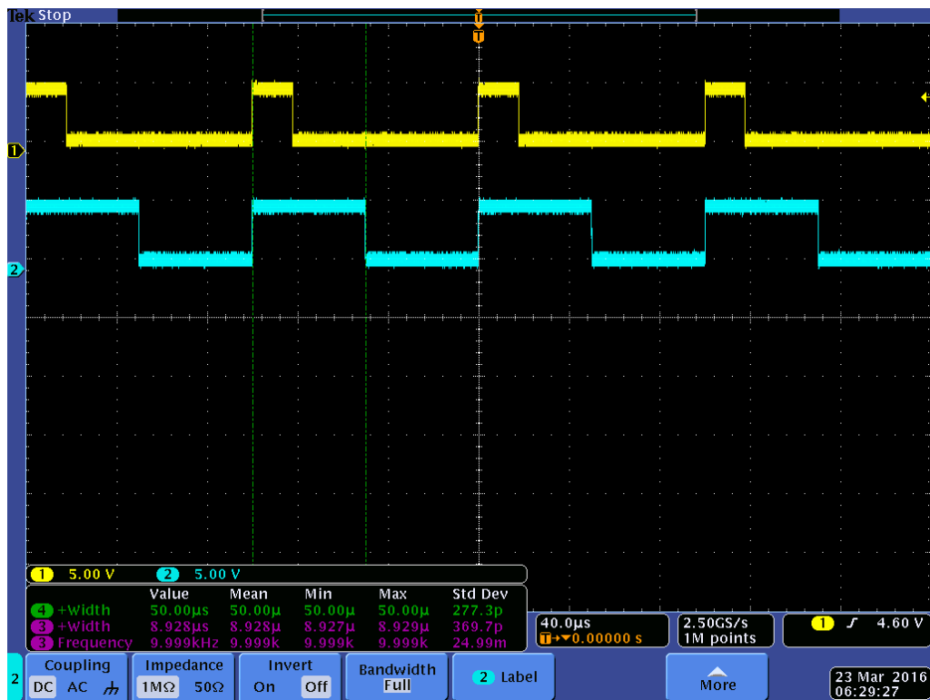
Figure 7. FTM0_CH0 and FTM0_CH2 input signals
