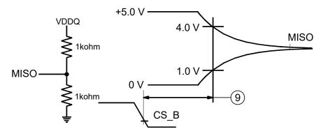
Figure 9. MISO loading for disable time measurement
