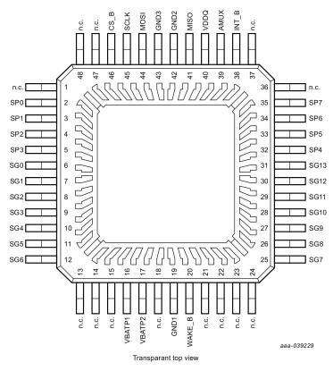
Figure 4. 33978 LQFP-EP pinout
