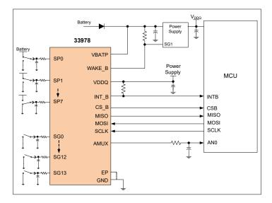
Figure 1. 33978 simplified application diagram
