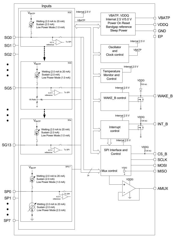
Figure 2. 33978 internal block diagram
