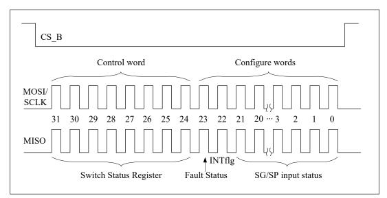
Figure 19. First SPI operation (after POR)
