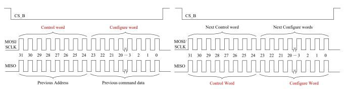
Figure 20. SPI write operation
