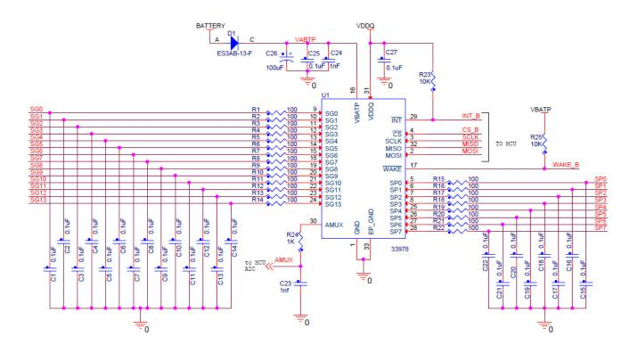
Figure 24. Typical application diagram
