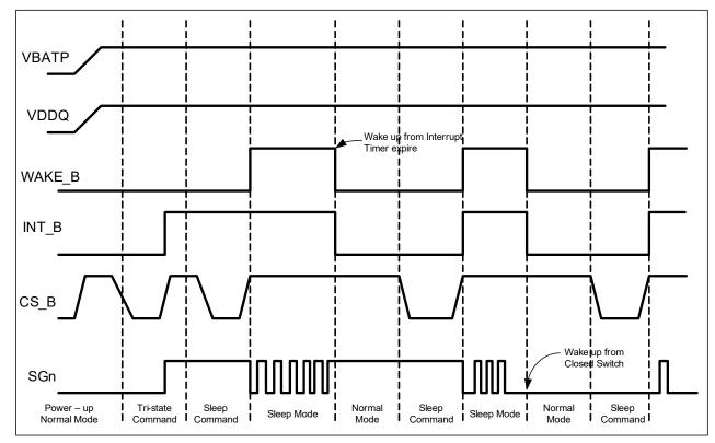
Figure 16. Low-power mode to normal mode operation
