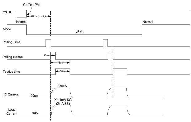
Figure 15. Low-power mode typical timing
