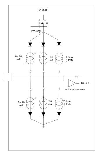
Figure 18. SP block diagram
