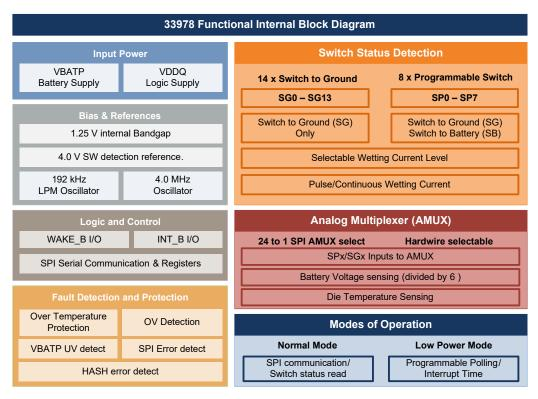
Figure 11. Functional block diagram
