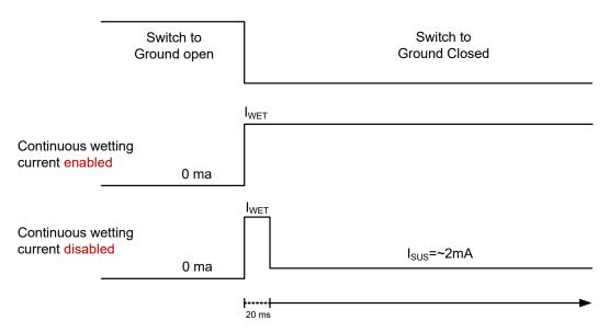
Figure 23. Pulsed/continuous wetting current configuration
