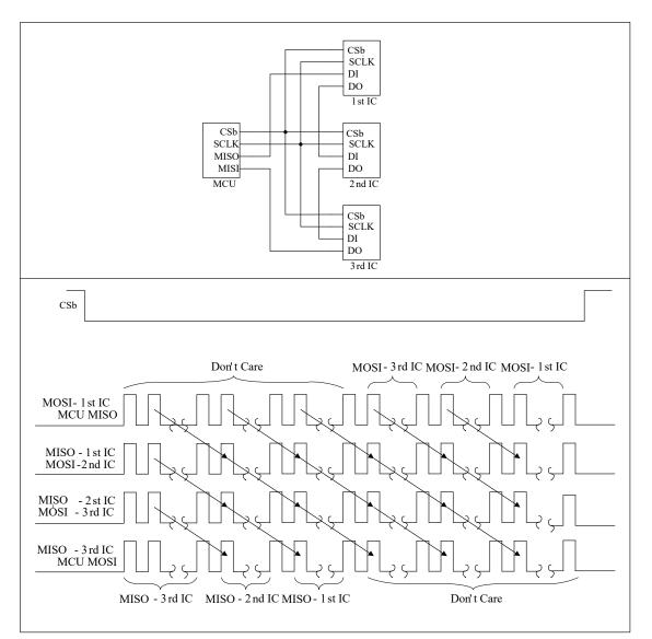
Figure 22. Daisy chain SPI operation
