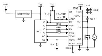
Figure 21. Typical Application Diagram
