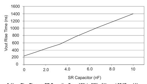
Figure 9.  $V_{OUT}$  Rise Time vs. SR Capacitor From 10% to 90% of  $V_{OUT}$  at 25 °C and  $V_{PWR}$  = 13 V
