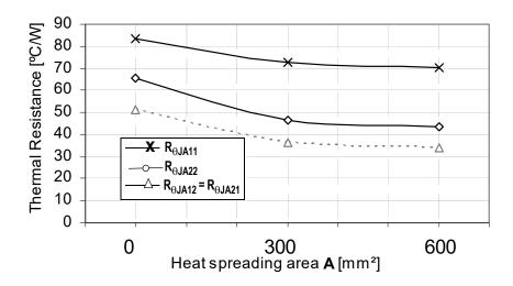
Figure 46. Device on Thermal Test Board  $\textbf{R}_{\theta \textbf{J} \textbf{A}}$
