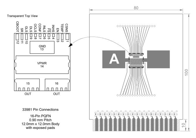
Figure 45. Thermal Test Board
