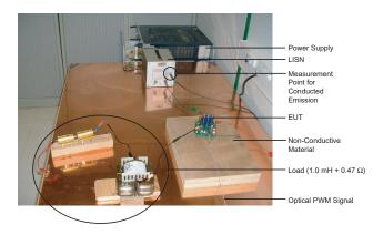
Figure 26. Conducted Emission Test Setup
