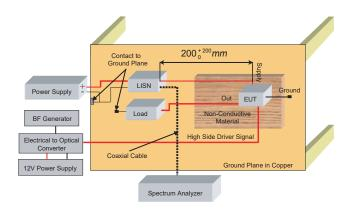
Figure 23. Test Bench for Conducted Emission
