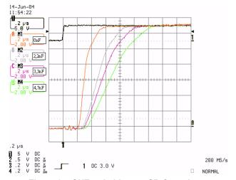
Figure 37. OUT switching vs. SR Capacitor
