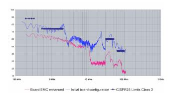
Figure 30. Conducted Emission Spectrum for 33981
