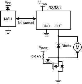
Figure 11. Reverse Battery Protection
