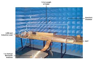
Figure 31. Radiated Emission Test Set-up
