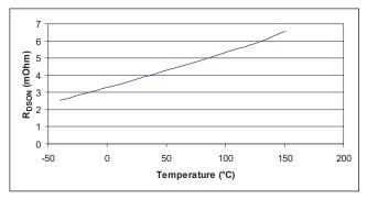
Figure 35. R<sub>DS(ON)</sub> vs. Temperature
