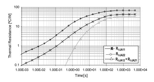
$\label{eq:Figure 47.} Figure \ 47. \ Transient \ Thermal \ Resistance \ R_{\theta JA},$   $\ 1 \ W \ Step \ response, Device \ on \ Thermal \ Test \ Board \ Area \ A = 600 (mm^2)$
