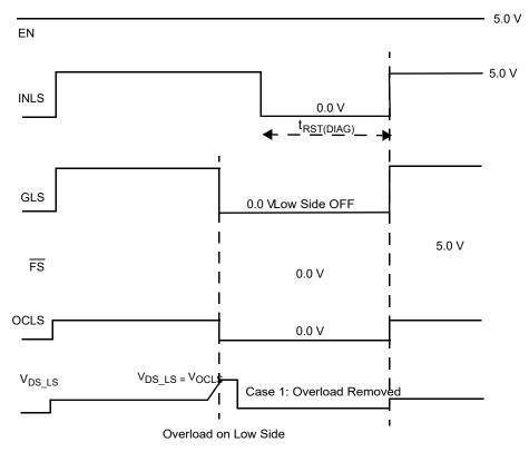
Figure 13. Overload on Low Side Gate Drive, Case 1
