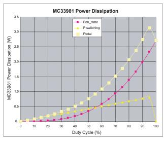
Figure 40. Power Dissipation (Pon and Pswitching) vs.
