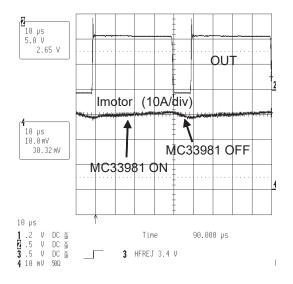
Figure 22. Current and Voltage waveforms
