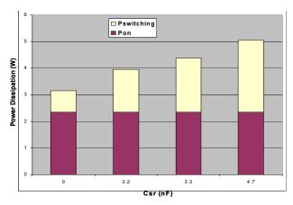
Figure 41. Power Switching vs. SR Capacitor
