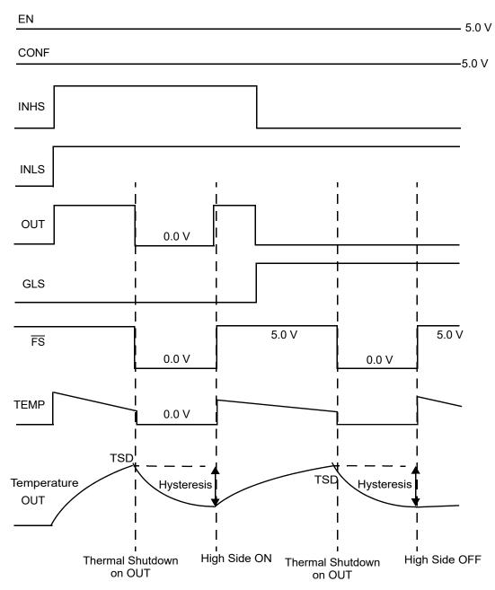
Figure 12. Over-temperature on Output
