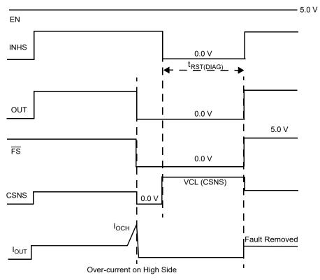
Figure 15. Over-current on Output
