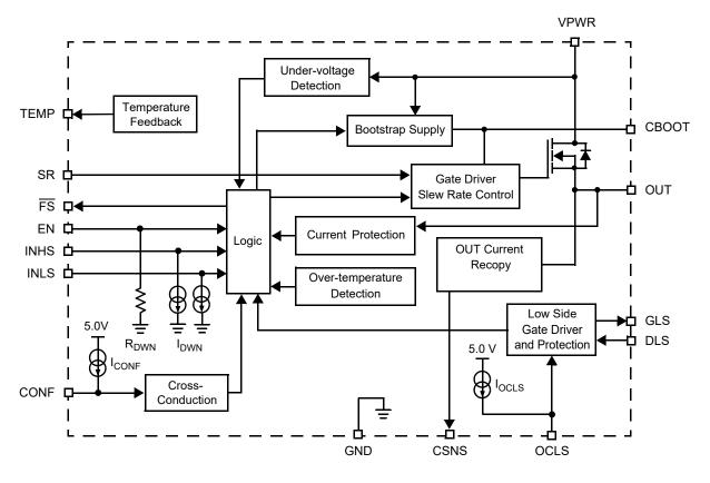
Figure 2. 33981 Simplified Internal Block Diagram
