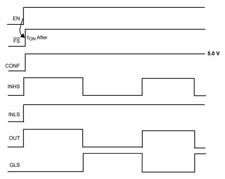
Figure 5. Normal Mode, Cross-Conduction Management
