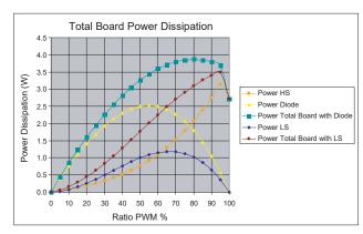
Figure 42. Total Board Power Dissipation
