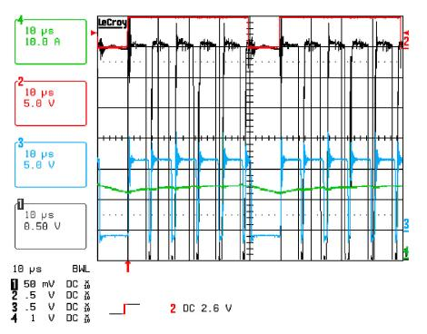
Figure 16. High Side Over-current
