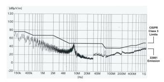
Figure 32. Radiated Emission Spectrum for 33981
