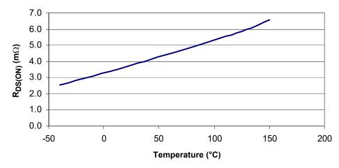
Figure 7. Typical  $R_{DS(ON)}$  vs. Temperature at  $V_{PWR}$  = 13 V
