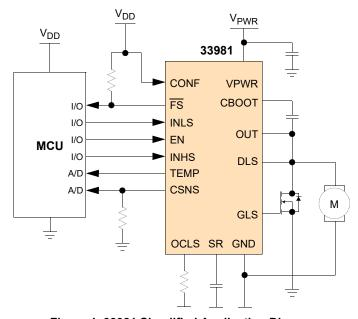
Figure 1. 33981 Simplified Application Diagram
