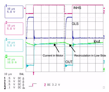
Figure 17. Cross-Conduction with Low Side
