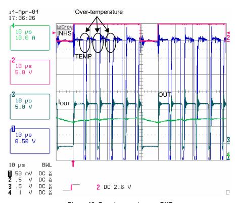
Figure 18. Over-temperature on OUT
