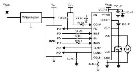
Figure 20. 33981 Typical Application Diagram
