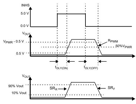
Figure 4. Time Delays Functional Diagrams
