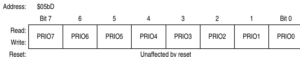
Figure 11-14. Transmit Buffer Priority Register (TBPR)
