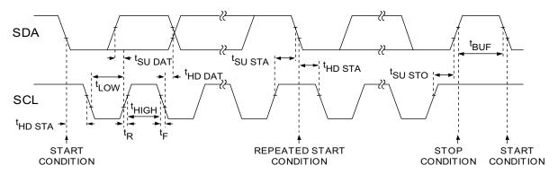
Figure 5. Wire Serial Interface Timing Details
