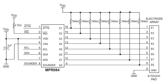
Figure 4. Recommended System Connections Schematic
