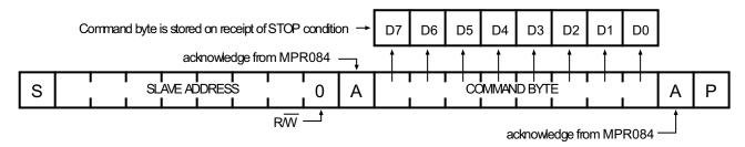
Figure 10. Command Byte Received
