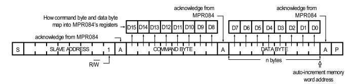
Figure 12. 'n' Data Bytes Received
