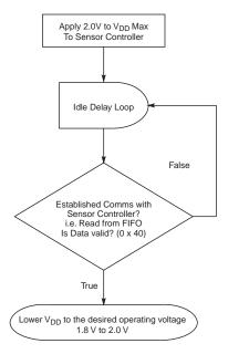
Figure 13. Low Voltage (1.8 V - 2.0 V) Power-up Sequence
