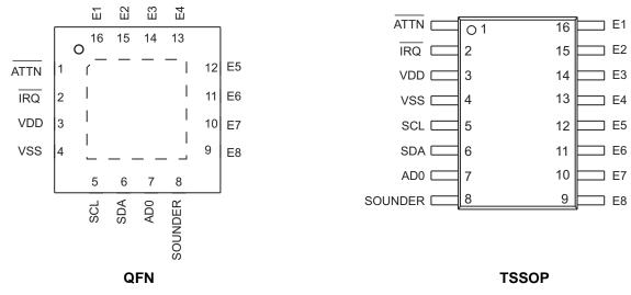
Figure 3. Package Pinouts
