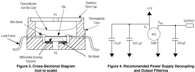
and Output Filtering (For additional output filtering, please refer to Application Note AN1646.)
