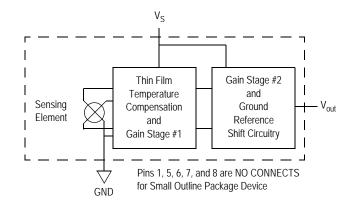
Figure 1. Fully Integrated Pressure Sensor Schematic
