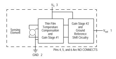
Figure 1. Fully Integrated Pressure Sensor Schematic
