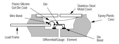
Figure 3. Cross-Sectional Diagrams (not to scale)
