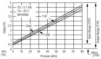
Figure 2. Output versus Pressure Differential
