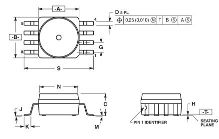
NOTES: 1. DIMENSIONING AND TOLERANCING PER ANSI Y14.5M, 1982. 2. CONTPOLLING DIMENSION: INCH. 3. DIMENSION A AND B DO NOT INCLUDE MOLD PROTRUSION. 4. MAXIMUM MOLD PROTRUSION 0.15 (0.006). 5. ALL VERTICAL SURFACES 5' TYPICAL DRAFT.
