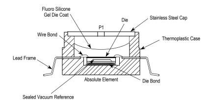
Figure 2. Cross Sectional Diagram SOP (not to scale)
