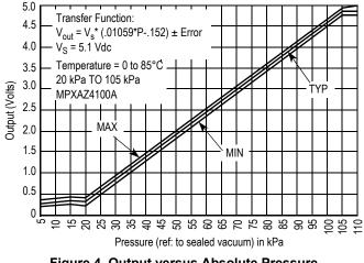
Figure 4. Output versus Absolute Pressure
