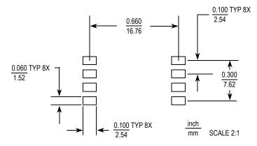
Figure 5. SOP Footprint (Case 482)
