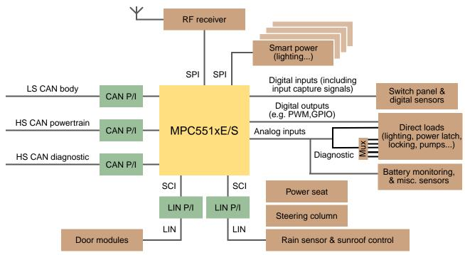
Figure 1. Body Controller Application Example
