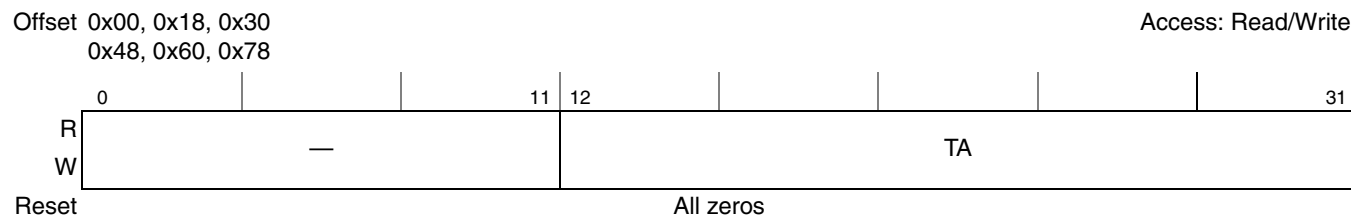
Figure 22-2. PCI Outbound Translation Address Registers (POTAR n )
