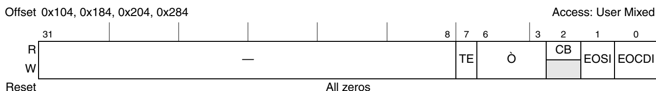
Figure 14-11. DMA Status Register (DMASR n )
