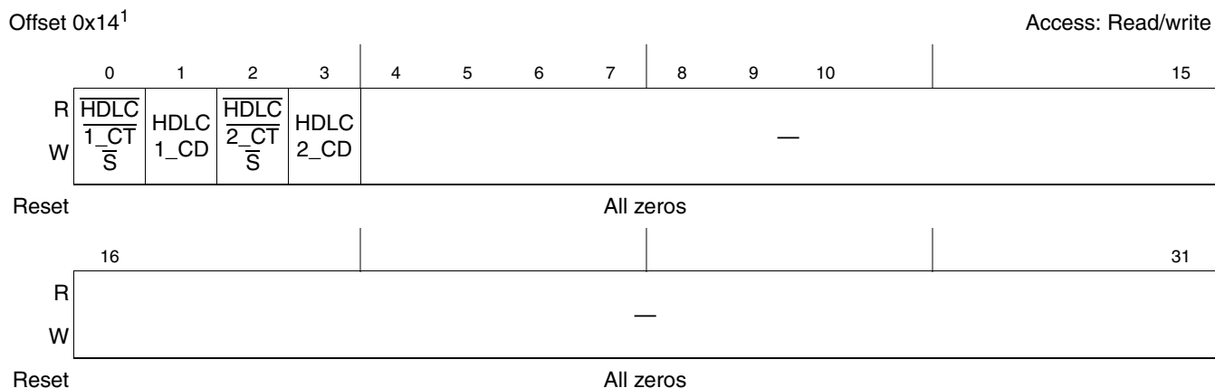
Figure 9-29. QUICC Engine Ports Interrupt Control Register (CEPICR)
