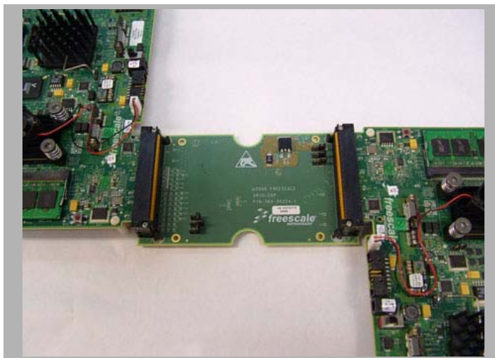
Figure 6-3. Two MSC8144ADS Boards Connected, Back-to-back
