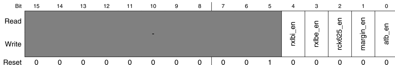
lane0_RX_ANA_CONTROL field descriptions
