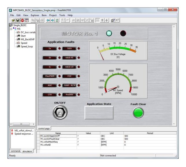
The HTML-based data visualization area. The user can provide any collection of ActiveX-based instrumentation to create custom visual dashboards as complex or elegant as desired.
