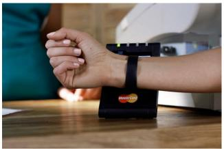
More specifically, the initiative makes it much easier to add the security functions needed to protect an NFC payment. NFC payments use a microcontroller-based circuit, called a secure element, to safeguard payment information and conduct the NFC transaction in a secure way. The secure payment functions are then added to the companion app that's used by, for example, a wristband, so the wristband can start making payments.
