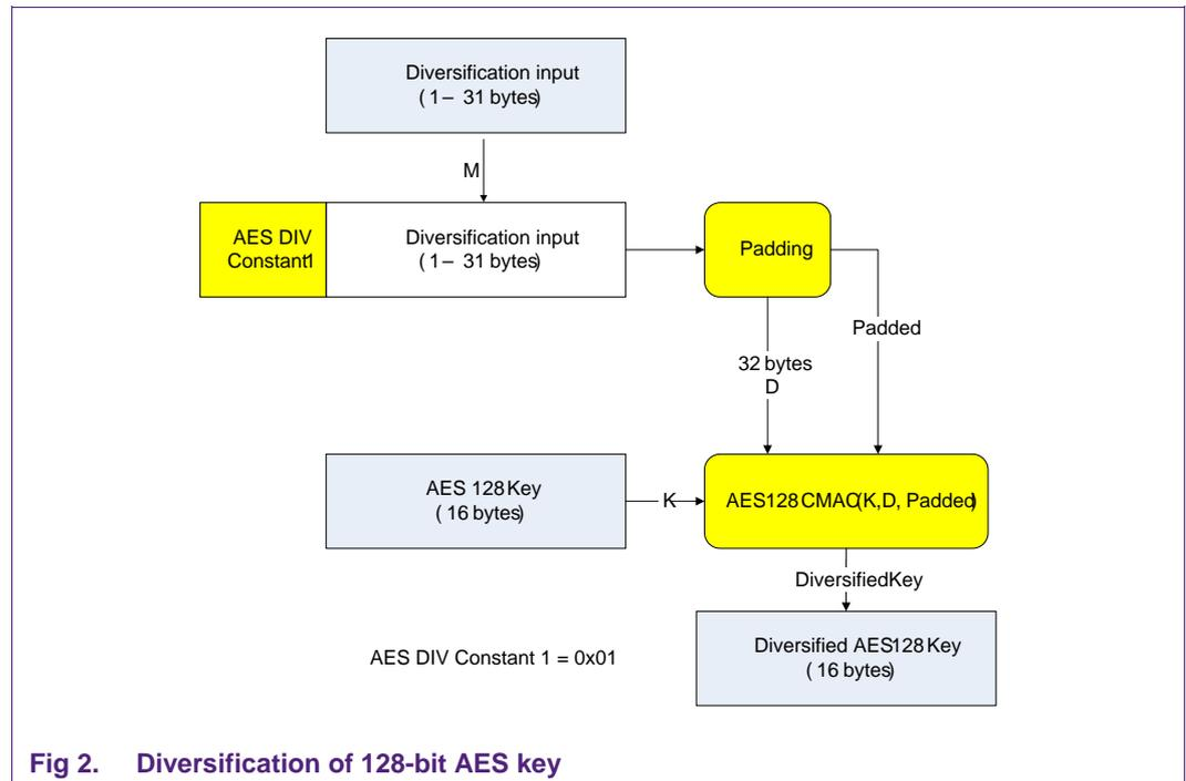
Fig 2. Diversification of 128-bit AES key
