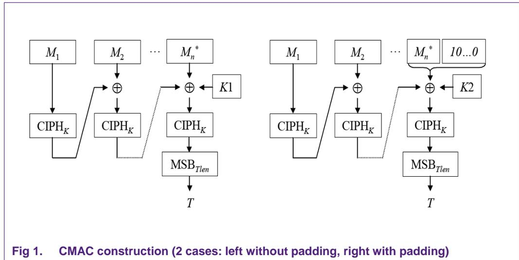
Fig 1. CMAC construction (2 cases: left without padding, right with padding)
