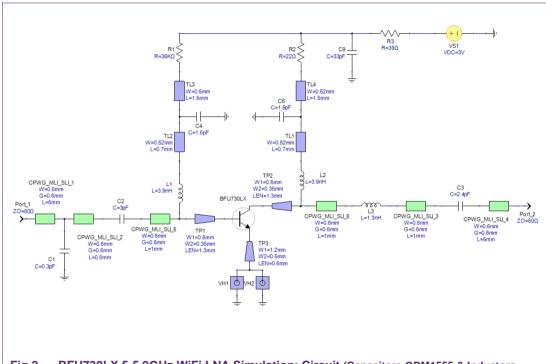
Fig 2. BFU730LX 5-5.9GHz WiFi LNA Simulation: Circuit (Capacitors GRM1555 & Inductors LQP15)
