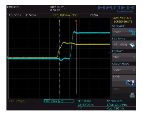
3.0 V rms, 1 kHz and 50% duty cycle pulse applied on VCC pin, measured from 50% of input pulse to 100% of max. output power
